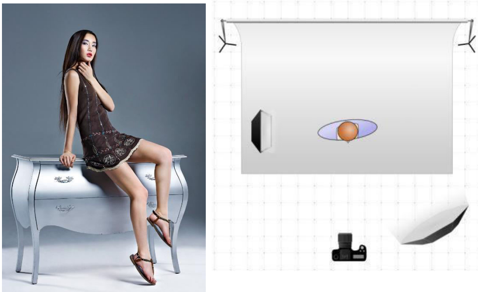
Fig.No.1 – Image showing the Lighting Setup for Catalogue Shoot.
